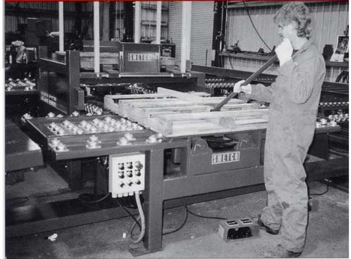
The "Palleturn" pallet repair table aids in pallet inspection, repair, and transfer to the stacker. 360 Degree ball transfer units are mounted on the table surface, allowing pallets to be easily pushed or rotated. The pallet hold-down clamp holds the pallet down while the operator removes boards. The "Palleturn" flipper arms help turn the pallet over.
