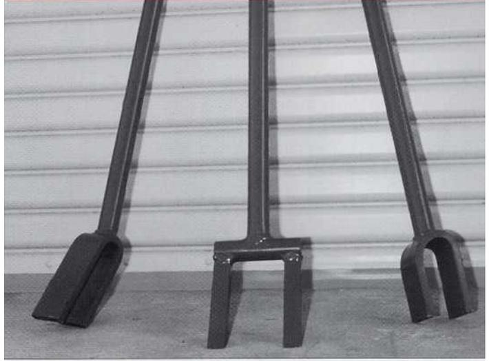
Smetco Pallet Repair Tools are designed to handle a variety of board removal problems. There are three styles included with each system.
