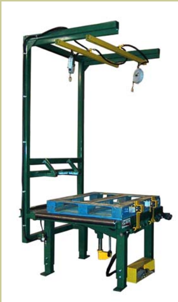
Block Repair Table
